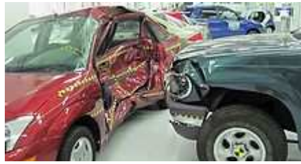
A crash test by the Insurance Institute for Highway Safety shows the damage to a compact Ford Focus struck by a Ford Explorer SUV
