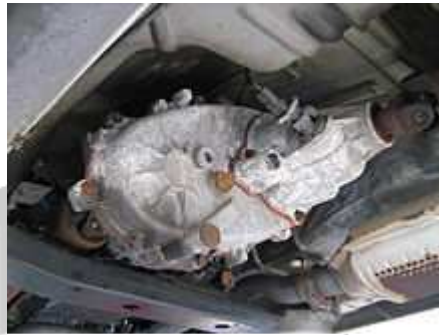
Center transfer case sending power from the transmission to two output shafts: to the rear axle (visible on the right) as well as to the front axle (on the left side)
