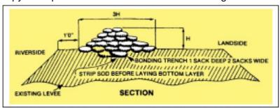
Stamp each bag in place, overlap sacks, maintain staggered joint placement, and tuck in any loose ends. Use the following table to estimate the number of bags required:
