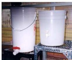
What you now have is an automatic lye water machine. Because the system is "closed," rain water cannot dilute the lye solution, but rain can be used as the source of water for the ashes, so lye water can be made in the winter. During heavy winter rains, a board can be placed over all but the first foot or so of the gutter, which will limit the amount of water intake and still allow what rain falls into the first foot to filter through all of the ashes to the exit down spout.
