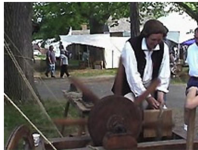
This foot powered machine turns a wheel; the spokes of the wheel beat the fibers as they are clustered in a bundle.
