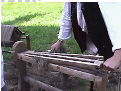
After soaked (or retted) flax has dried, the stem is cracked on a tool called a flax break. Small bundles of flax are placed across the lower wooden blades; the upper blades break the outside chaff.
