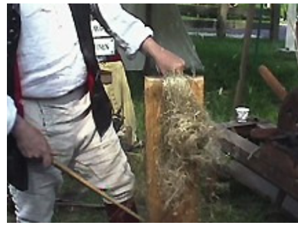
The scutching knife is struck against a vertical wooden board to remove the loose pieces of stem from the fiber.
