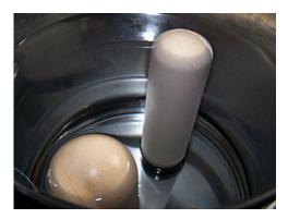
The advantages of this unit are its ease of operation, huge capacity and superior filters. Disadvantages are cost and the fact that it is not effective against viruses so boiling is still advised if viruses are suspected.
