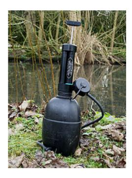
This is one of my favorite units. It has course and fine filters and iodine resin built in. It also nests neatly into the mouth of a 58 pattern water bottle. Water is pumped into a long tune (with course stuff filtered out through the pre filter)
