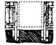
the distance between the inside of the two gates posts to ensure the gate can swing freely. After the gate has been constructed properly for the space desired, attach the hinges and gate latch. If you desire a stop, nail a piece of fencing material to the latch post.
