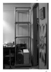
Adam Byers got creative and constructed a custom shelf on casters made from Kee Klamp fittings, fence post and some plywood. Instructions to build this project are posted on <a href="http://adambyers.com/kee-klamp-shelf-not-so-much-on-the-cheap/">http://adambyers.com/kee-klamp-shelf-not-so-much-on-the-cheap/</a>) and on <a href="http://www.instructables.com/id/Kee-Klamp-Shelf/">http://www.instructables.com/id/Kee-Klamp-Shelf/</a>). Great project Adam, thank you for sharing it with us.
