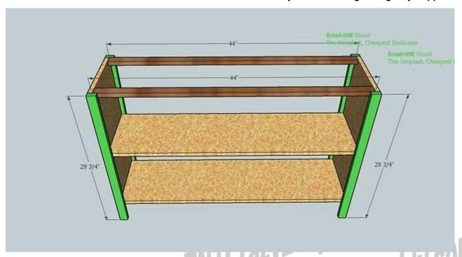
3. **Legs**. Nail the legs, D (Green) in place, as shown above. Keep outside and top edges flush. Make sure you nail through the legs into the shelves and the top support, C.
