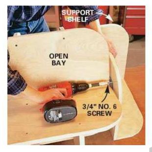
7. Center the 3-in. lazy susan at the rotation center on the support shelf. Screw the top ring of the lazy Susan to the support shelf with the 3/4-in. screws.
