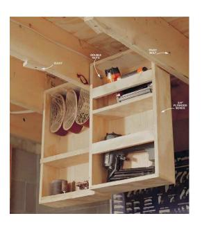
Eke out every cubic inch of storage in a basement shop with pivoting boxes that hang between the ceiling joists. When a drawer is down, you have easy access to its contents. Use glue and 1-5/8 in. drywall screws to hold together the boxes, then customize shelving for whatever you want to store.
