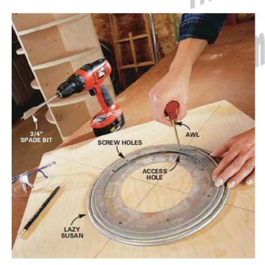
4. Center the 12-in. lazy Susan on the base. Align the screw holes on the top and bottom rings. Locate the access hole in the lazy Susan and mark its location on the plywood with an awl or nail. Remove the lazy Susan and drill a 3/4-in. hole at the mark. Center the lazy Susan again, aligning the access hole to the hole drilled in the plywood, and fasten the bottom ring to the base with 3/4-in. No. 6 flat head screws.
