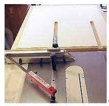
Grooves were routed in the top for clearance of the miter guide bars. I also rounded over all
