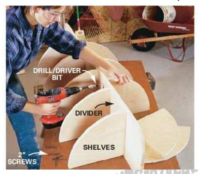
2. Measure and mark the shelf locations on the dividers, spacing them anywhere from 10 to 14 in. apart. Align the shelves with these marks, then predrill and screw the shelves to the two narrow dividers with 2-in. drywall screws. A drill/driver bit speeds this process (\$10 at home centers).
