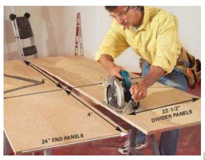
1 Rip one 8-ft. long, 24-in. wide length of 3/4-in. plywood for the end panels and 22-1/2 in. widths for each divider panel. Cut the panels to 4-ft. lengths.
