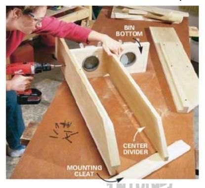
**5.** Predrill and screw the center divider to the bin bottom with 2-1/4 in. Trim head screws. Then add the sides, bottom, and top. Next attach the back and the top half of the cleat with 1-1/4 in. screws.
