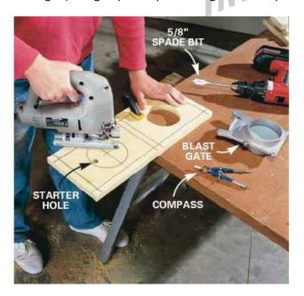
2. Lay out the bays on the bin bottom using Fig. D as a guide. Find the center of each bay and draw the circular cutout for the blast gates with a compass. Drill a 5/8-in. starter hole and cut out the openings with a jigsaw.
