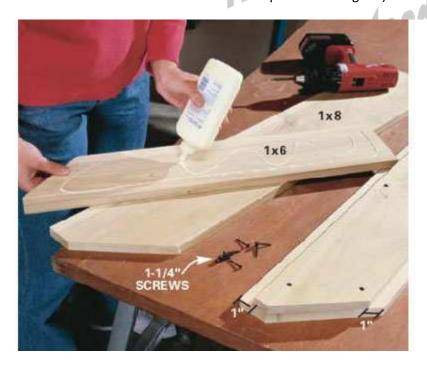
**4.** Glue and screw the two-piece sides together (Fig. D). Use 1-1/4 in. screws and predrill with a 1/8-in. bit to avoid splitting the wood.
