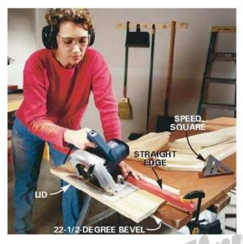
Set your saw to an angle and rip the lid (22-1/2 degrees) and mounting cleat (45 degrees). Clamp or screw the boards to your workbench and use a straight guide for these cuts. Cut the other parts to length (see cutting list and fig. D) using a speed square as a guide to keep the cuts square.
