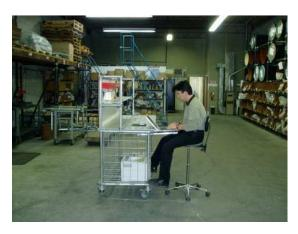
The guys over at Kee have constructed this awesome work cart for use in one of their warehouse locations. You can see that it has storage below for boxes, a place to store tools, a place to pack boxes, and even a platform for a laptop computer. To top it all off it's on casters so that it can be rolled around to different locations, infill panels to enclose the space below and a nice stainless steel desktop. Great project!
