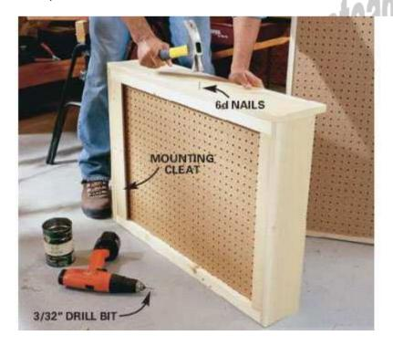
3. Measure and cut the 1x6 frame boards to fit around each panel. Glue and nail the top and bottom first, then the sides, to the 1x2 spacers with 2-in. (6d) finish nails spaced every 8 in. Fasten the frame board corners with two nails and glue. Predrill all holes with a 3/32-in. drill bit to avoid splitting the wood.
