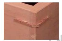
To add to the strength of the corners, I like to reinforce the corners (http://www.woodgears.ca/box\_joint\_alt/index.html ) by cutting a slot into them at 45 degrees, and then gluing a wood triangle into the slot. I do this after the main box is assembled, so there is no alignment issues. I stack three saw blades (http://www.sentex.net/~mwandel/workshop/dado.html ) to do this. After gluing the corner pieces in, I flush trim them.
