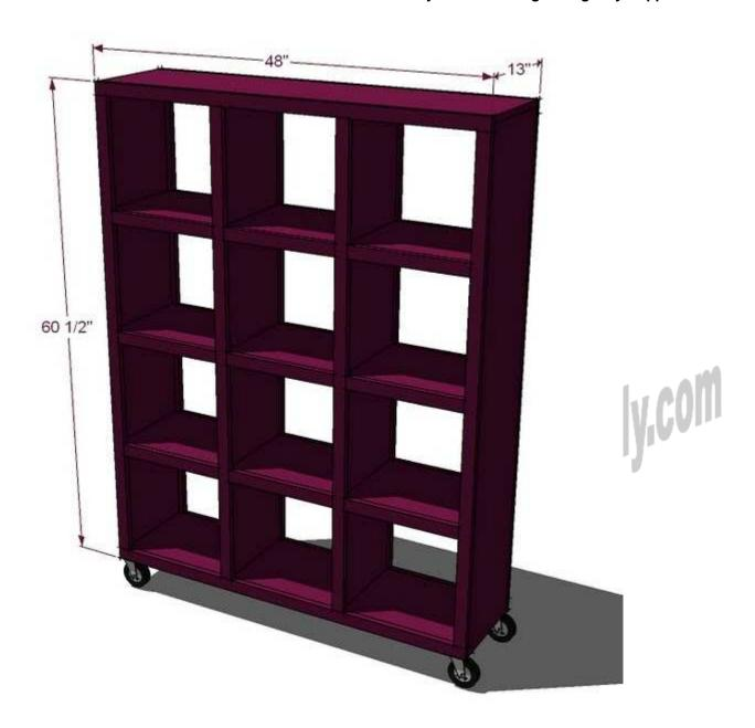
**Overall Dimensions are shown above.** Height without caster wheels is 60 1/2". Depth is 13" and width is 48". Caster wheels will add approximately 2 1/2" to the overall height. You can purchase different height caster wheels.
